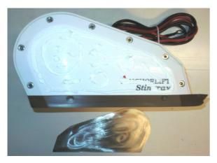
When alcohol has dryed apply glu on th windlass. Use polyurethan sealant. Sikaflex 11FC Sikaflex 290DC 3M Fast Cure 4200 or simmilar products.
